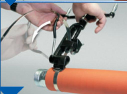
Pull on cutter lever, band is cut off to correct length.
