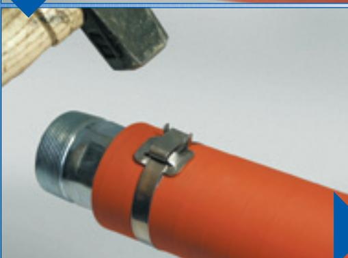
Hold stub of band with thumb, hammer it flat over bridge of buckle, complete clamp by hammering ears over stub.
