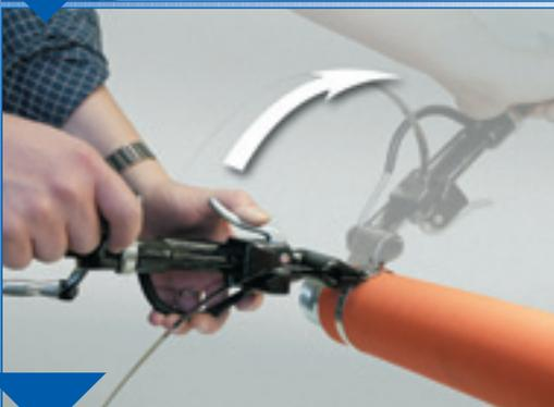
Place band in tool, push down on gripper with thumb, tension clamp by turning handle. Maximum tension is reached when band stops moving through buckle. When required tension has been applied, roll tool over buckle, at the same time reversing handle carefully approx. 1/2 turn to avoid breakage. There is no loss of tension, if handle is not reversed too much.
