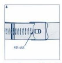
Locate the tongue of the buckle in the 4th slot of the band. Screw the band through using a hand or power tool.
